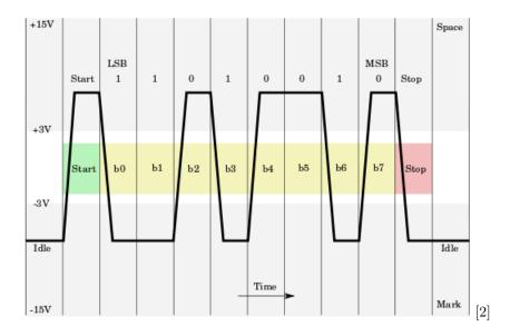
Instead, what we built in lab is an UART (Universal Asynchronous Receiver/-Transmitter). The UART protocol has the high idle states and non-reversed signaling at DC voltages. [3]
