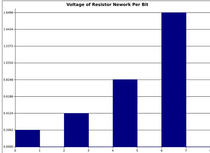
Where the LSB is on the left, and the MSB is on the right. To find any other combination of powered and grounded bits, simply add the voltages for the bits that are high (3.3v) to find the resultant  $V_{out}$ .
