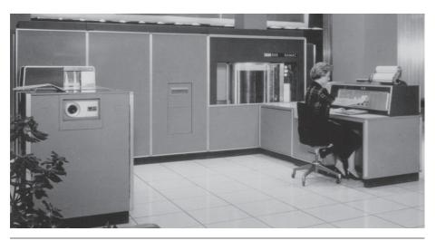
FIGURE 6.14.2 The RAMAC disk drive from IBM, made in 1956, was the first disk drive with a moving head and the first with multiple platters. The IBM storage technology Web site has a discussion of IBM's major contributions to storage technology.
